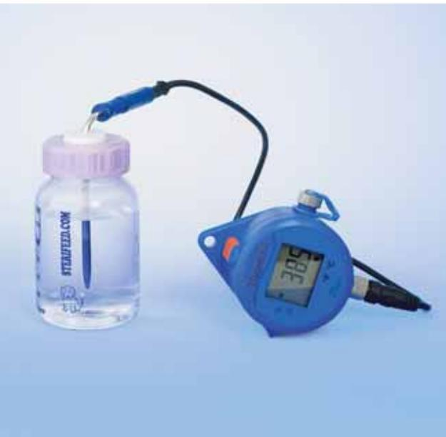
Dual programme selection to give specified temperature and times which are normally : 62.5°C x 30 minutes for Mothers' Milk. Rapid, precise refrigerated cooling of feeds to 4°C in approximately 30 minutes. Total cycle time is 90 minutes. This will depend on the temperature of the incoming hot water supply and ambient temperature.
